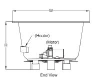
Note: Drain installation is non-standard. Vertical overflow connection requires offset.
